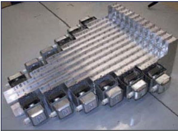
**Fig. 4** The installed magnetrons.
