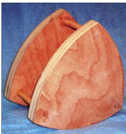
Fig. 1. A board placed on top of this wheel may be pulled along without any vertical movement taking place.
