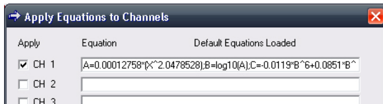
Figure 18 – First and second calibration equations entered into RSP.
